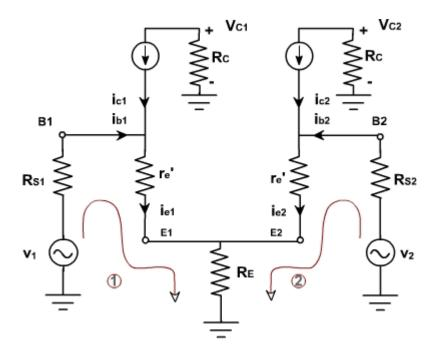
AC EQUIVALENTCIRCUIT FOR DUAL-INPUT BALANCED OUTPUT DIFFERETIAL AMPLIFIER
